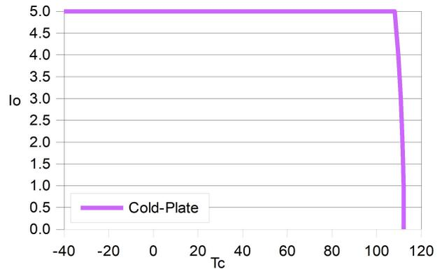
降额曲线(外加液冷板) ( $T_c = 120^{\circ}\text{C}/\text{OTP}$ )
